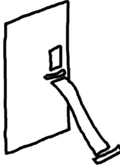
Figure 4.1: Using bracing to secure a door
